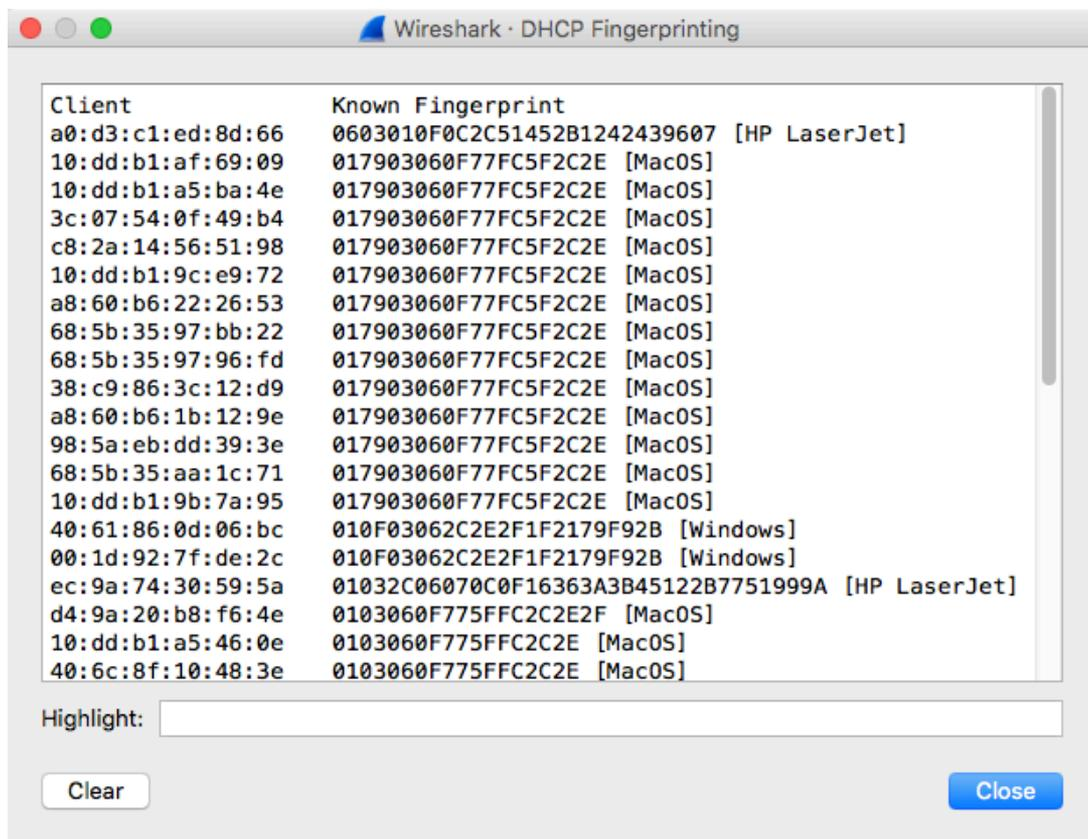
The image shows a screenshot of the Wireshark DHCP Fingerprinting window. The window title is "Wireshark · DHCP Fingerprinting". It contains a table with two columns: "Client" and "Known Fingerprint". The "Client" column lists MAC addresses, and the "Known Fingerprint" column lists the corresponding fingerprints and device models. At the bottom of the window, there is a "Highlight:" text box, a "Clear" button, and a "Close" button.
